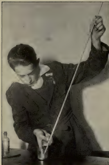
FIG. 153. Inverting the filled tube in the cup of mercury.
